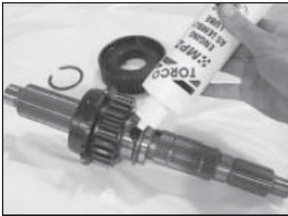
(Fig. 3A) New Main Output Shaft Assembly
