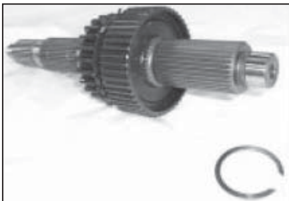
(Fig. 4A) (Large) Retaining Ring Installation
