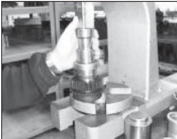
(Fig. 2A) Pull the Needle Bearings Out
